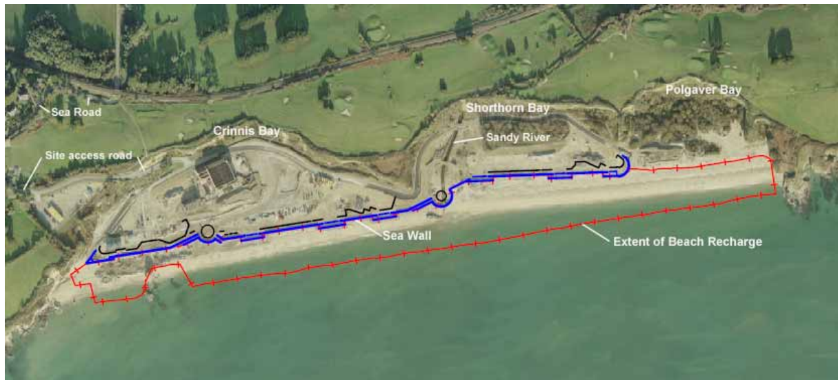
Figure 1 Aerial photo of Carlyon Bay with the proposed extent of the revised sea wall and beach recharge.
